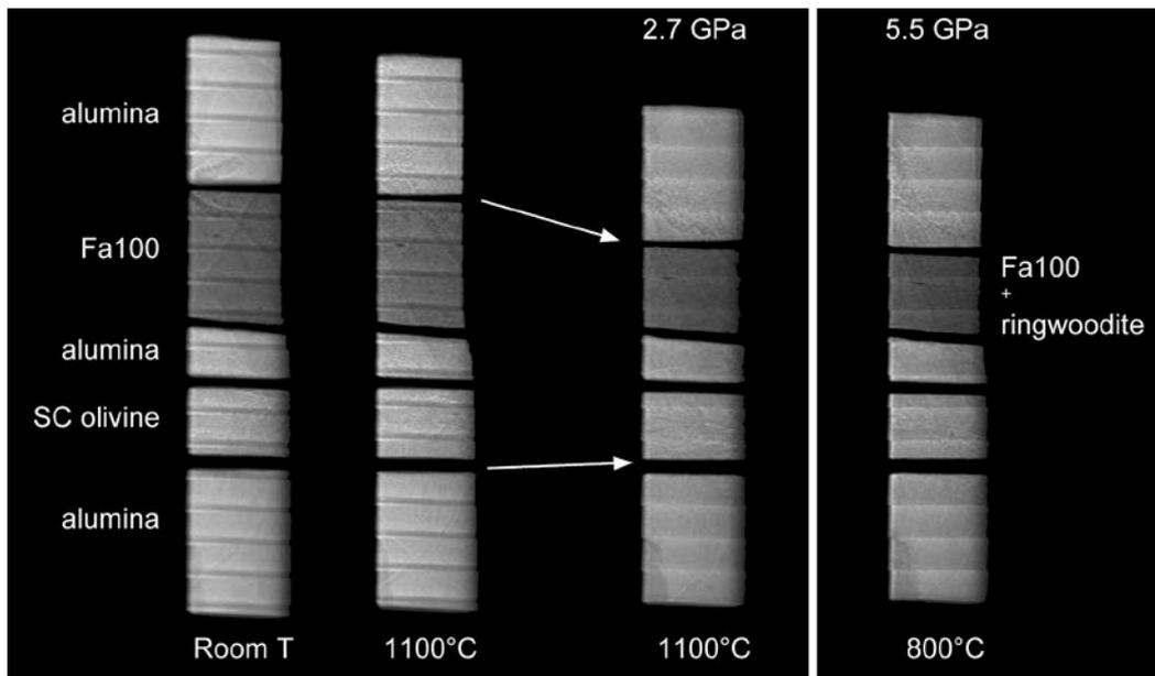
**Figure 2:** Top, x-ray radiographs of D-DIA compression column as seen through the front-anvils gap (~1 mm wide) after compression and during deformation at the indicated  $P$  and  $T$ . The image is composed of a series of 24 images (1x1 mm<sup>2</sup>) recombined together. The acquisition time is < 1 min. Note the (dark) Re foils indicating specimen ends.
