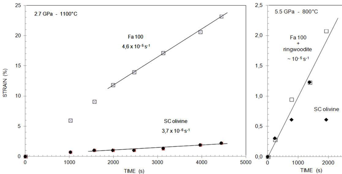
Bottom: specimen strain vs. time curves during the deformation episodes showed above; the slopes (values indicated) are specimen strain rates (indicated). Note that, at 2.7 GPa and 1100°C, steady-state conditions of deformation were achieved. See text for further explanation.
