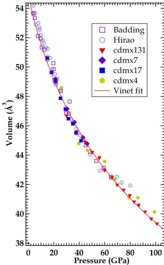
Figure 1 - Volume of dhcp-FeH as a function of pressure
