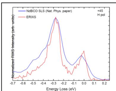
Figure 3. Antiferromagnetic NBCO Cu  $L_3$  RIXS. The red spectrum measured at ID32 shows a sharp magnon peak and the phonon as a shoulder of the elastic.
