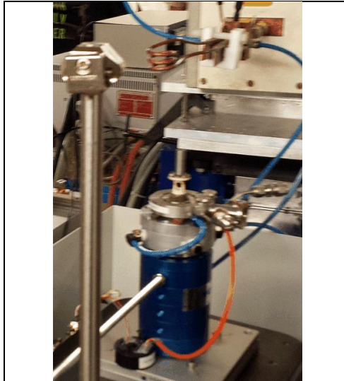
Figure 1 : slip ring mounted under the furnace (MRTOMO stage on ID19).
