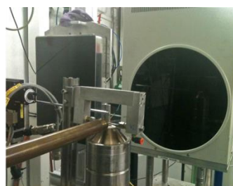
Figure 1: The setup for the in-situ studies of ceria based catalytic materials. This capillary setup also allows the use of different gases and use of different materials.
