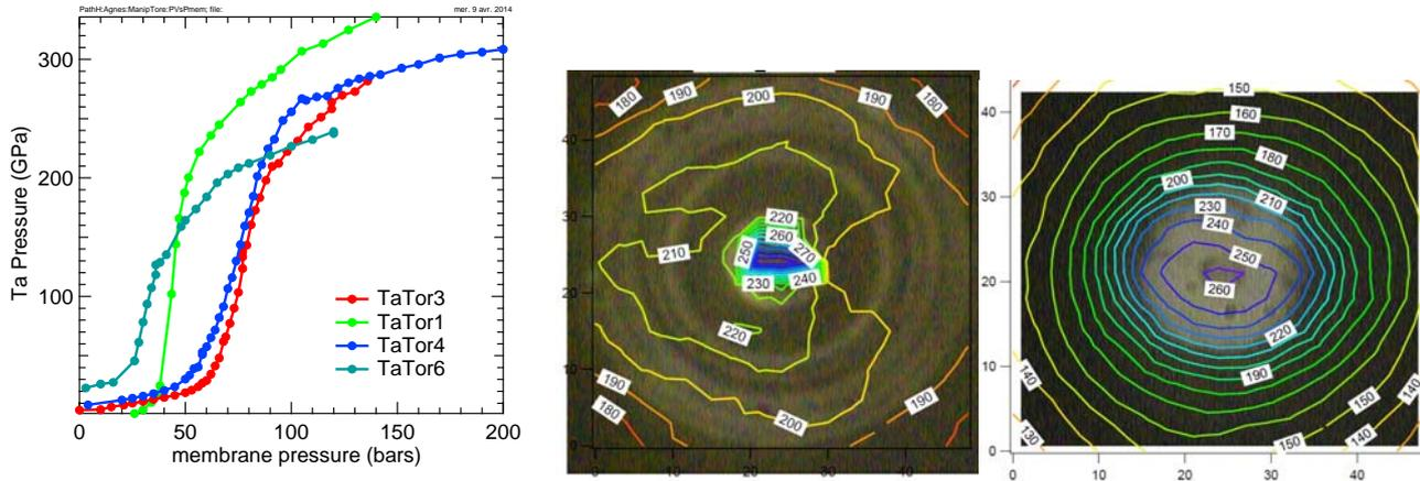
**Figure 2:** left: reached pressure, measured with tantalum equation of state, as a function of the membrane pressure which is proportional to the force applied on the back of the diamonds; center: pressure distribution map in run TaTor4 (pressure in GPa, position in microns); right: pressure distribution map in run TaTor3, diamonds with no tore (same units). The pressure maps are superimposed on photographs of the anvils culet.
