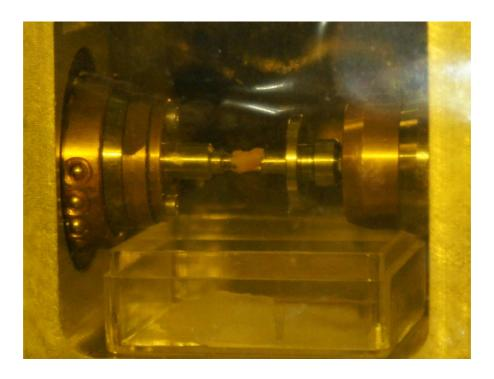
By doing so, time-lapse tomography with moderate temporal resolution of around 30 min per scan could be carried out on fresh, bio-regenerated bone. Hence, crack propagation could be studied in detail:
