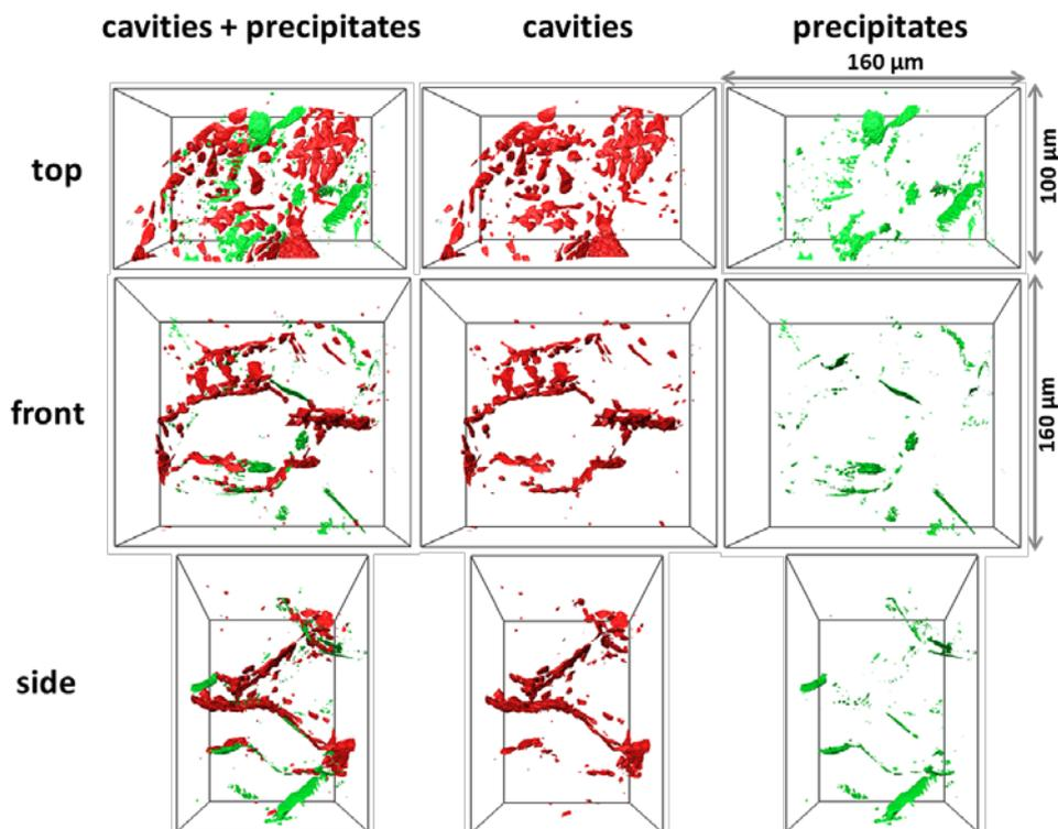
**Fig. 2.** (a) Spatial distribution of cavities and precipitates in a region of interest of the Fe-Au sample after creep at 550 °C and 60 MPa. The applied stress is normal to the top view.
