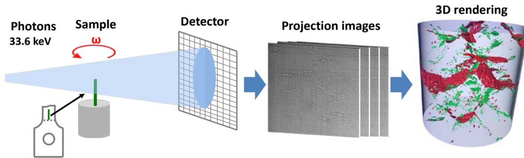
**Fig. 1.** Schematic diagram of the synchrotron X-ray holotomography imaging process. In the 3D rendering the precipitates and cavities are labelled in green and red, respectively, while the iron matrix is light grey.
