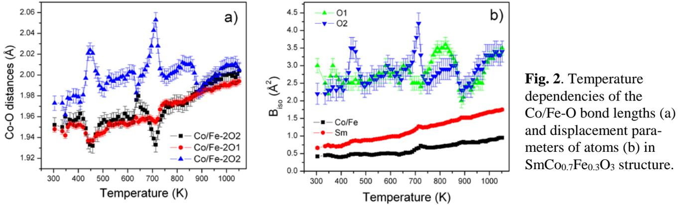
**Fig. 2.** Temperature dependencies of the Co/Fe-O bond lengths (a) and displacement parameters of atoms (b) in  $\text{SmCo}_{0.7}\text{Fe}_{0.3}\text{O}_3$  structure.
