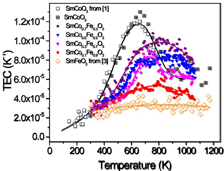
**Fig. 3.** Temperature dependence of average linear thermal expansion coefficients of  $\text{SmCo}_{1-x}\text{Fe}_x\text{O}_3$  series ( $x = 0, 0.3, 0.5, 0.7$  and  $0.9$ ) in comparison with the literature data for the “pure”  $\text{SmCoO}_3$  and  $\text{SmFeO}_3$ .
