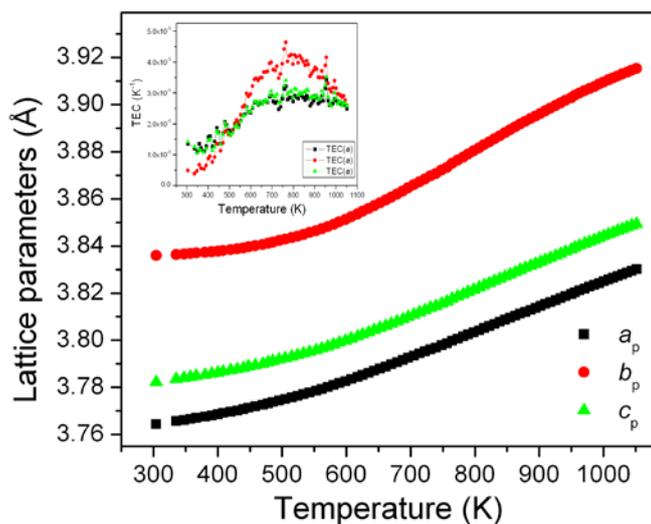
**Fig. 1.** Temperature dependence of the normalized cell parameters and thermal expansion coefficients (TEC) (insert) of  $\text{SmCo}_{0.7}\text{Fe}_{0.3}\text{O}_3$ .
