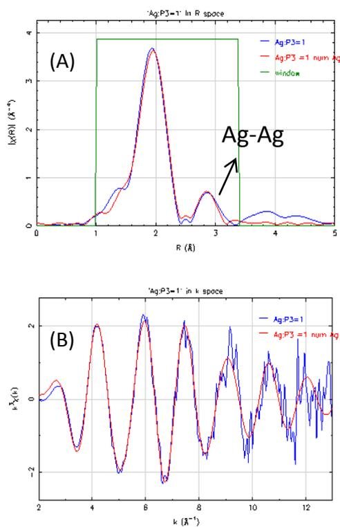
**Figure 1:** (A) Fourier-Transformed Ag K-edge EXAFS signal of the AgP3 complex (blue) and its R-space fit based on the Ag<sub>2</sub> digonal planar model. (B) EXAFS signal (blue) and its best-fitting curve (red) in the k-space.
