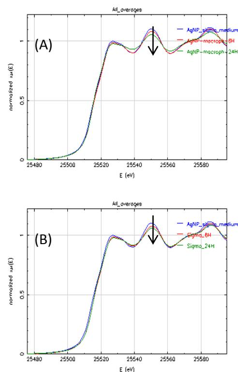
**Figure 3:** Ag K-edge XANES spectra of raw Ag-NP (commercial product from Sigma, blue line) and cellular models exposed to Ag-NP for 6 hours (red) and 24 hours (green). Cell lines were either macrophages (A) or hepatocytes (B).
