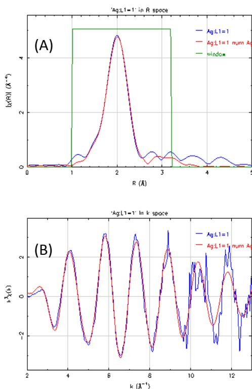
**Figure 2:** (A) Fourier-Transformed Ag K-edge EXAFS signal of the AgL1 complex (blue) and its R-space fit based on the Ag<sub>3</sub> trigonal planar model. (B) EXAFS signal (blue) and its best-fitting curve (red) in the k-space.
