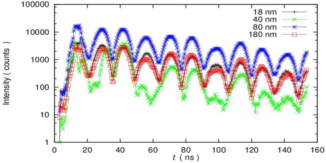
Fig. 1: The nuclear forward scattering spectra obtained on 20, 40, 80 and 180 nm diameter Fe nanowires with  $k_{\perp}$ NW.
