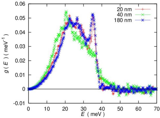
Fig. 2: Fe specific DOS measured in 20, 40 and 180 nm diameter Fe nanowires with  $k_{\perp}$ NW
