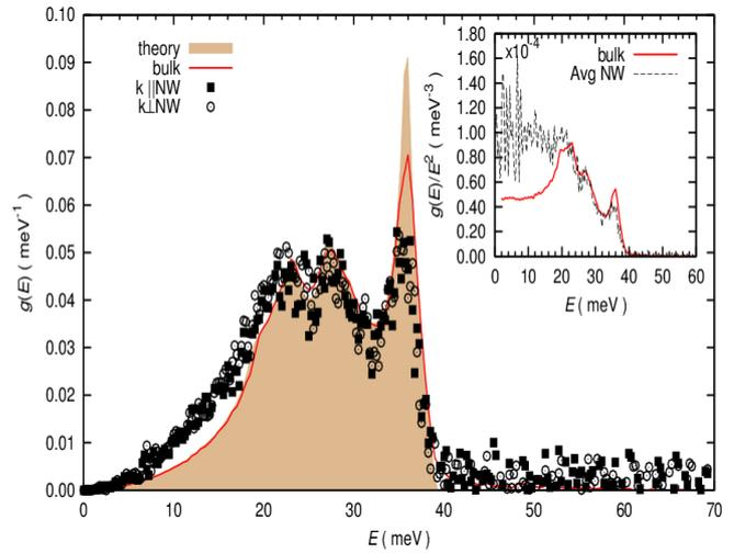
Fig. 3: Fe specific DOS measured in two geometries on 20 nm diameter Fe NW, with  $k_{\parallel}$ NW and with  $k_{\perp}$ NW, and comparison to similar measurements on bulk single crystals and theoretical calculations. Inset: comparison of the Debye level between bulk sample and NW.
