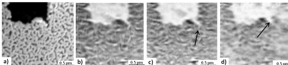
Figure 1: Np-Au on a SiN membrane studied by SEM (SE contrast) and ptychography at different annealing steps with a flow of 3 ml / min synthetic air. a) Ex situ SEM image in SE contrast before any thermal treatment, b) phase contrast image of the same area in the ptychographic measurement at room temperature, c) phase contrast image at a power of 59 mW d) phase contrast image at a power of 130 mW.
