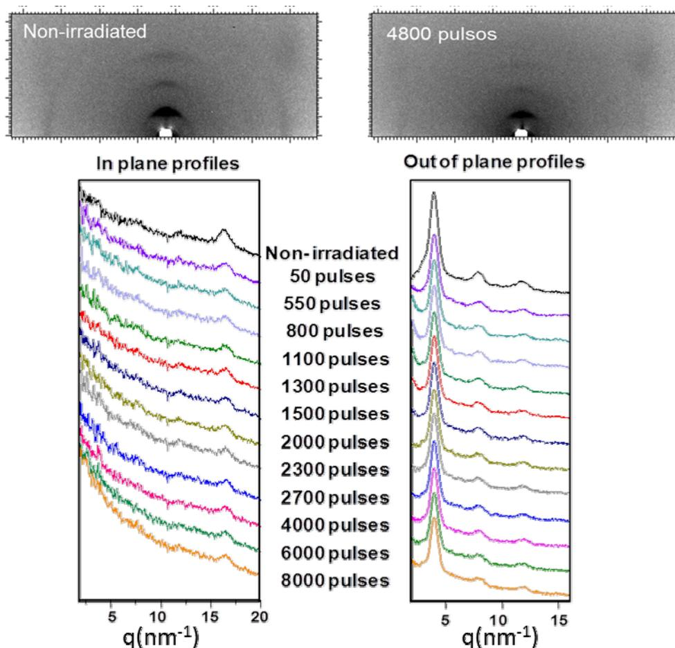
**Fig. 2.** (Upper panel) 2-D GIWAXS patterns of P3HT before and after irradiation with 4800 laser pulses at  $26 \text{ mJ/cm}^2$ . (Lower panel) In situ GIWAXS patterns obtained during laser irradiation at  $26 \text{ mJ/cm}^2$  of a P3HT thin film at different number of pulses. In plane (left) out of plane(right).
