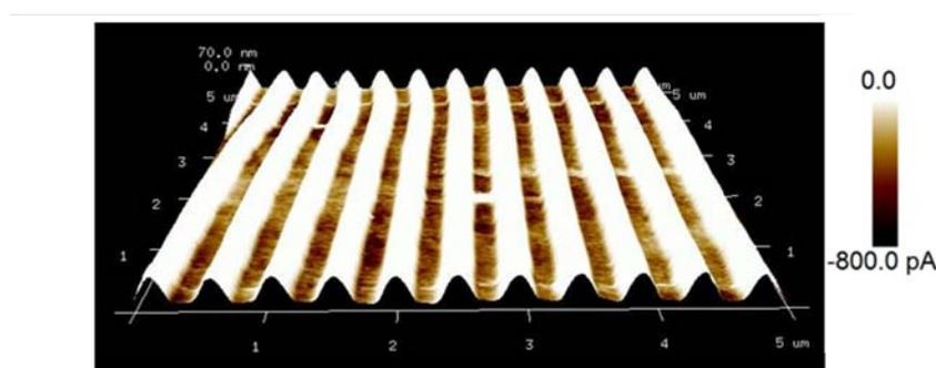
Figure 3. Overlapped AFM height image (contact mode) and C-AFM measured at constant bias of -5 V for a LIPSS of P3HT.
