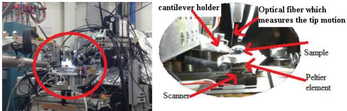
Figure 1: Left) AFM mounted at ID03. Right) zoom on the central part of the AFM: the sample holder on the top of the scanner, including the Peltier element. The cantilever holder and the fiber holder are visible on the top.
