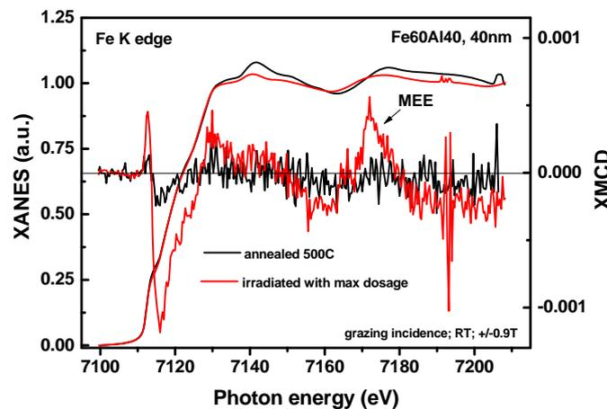
Fig.1 XANES (left scale ) and XMCD (right scale) spectra measured at Fe K edge for annealed (ordered, B2) and irradiated with max fluence (disordered, A2)  $\text{Fe}_{60}\text{Al}_{40}$  samples of 40nm thickness
