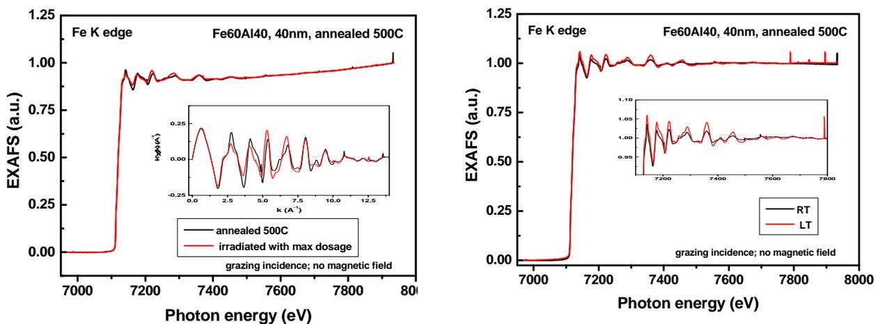
Fig.2 EXAFS spectra at Fe K edge measured for annealed (B2) and irradiated (A2) samples at RT (left); for annealed (B2) sample at RT and LT (100K) (right)
