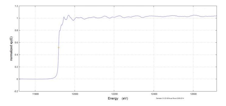
Figure 1: Raw EXAFS data for AuNPs/3MPS/TG sample (Au/thiols stoichiometry = 1/4/6).
