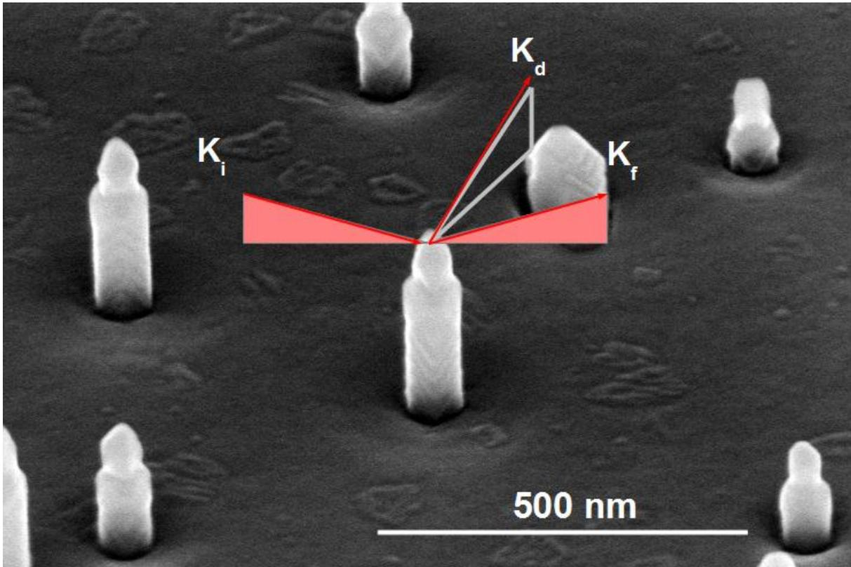
**Figure 1:** SEM image of GaAs/Fe<sub>3</sub>Si core/shell NWs and islands grown by molecular beam epitaxy on a Si(111) substrate at a substrate temperature of  $T_S = 200^\circ\text{C}$ . The geometry of XRD in grazing incidence geometry is sketched on top of the micrograph.  $K_i$ ,  $K_f$ , and  $K_d$  are the wave-vectors of the incident, reflected, and diffracted beams, respectively.
