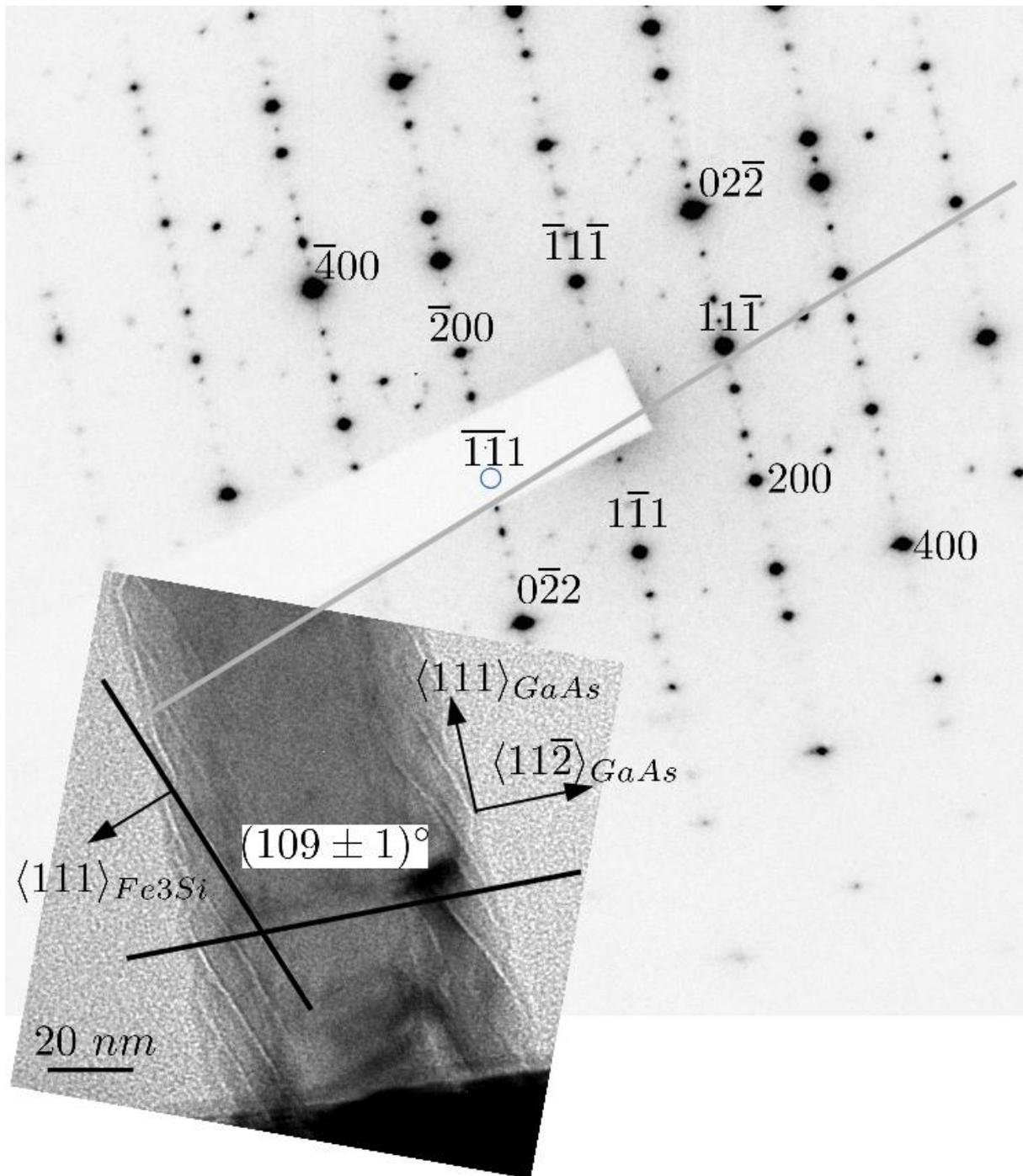
**Figure 4:** Multi-beam bright-field TEM micrograph and the corresponding SAD pattern illustrating the orientational relationship of a GaAs/Fe<sub>3</sub>Si core/shell NW. The straight line near the (11-1) reflection is oriented perpendicular to the nanofacets of Fe<sub>3</sub>Si visible in the corresponding micrograph.
