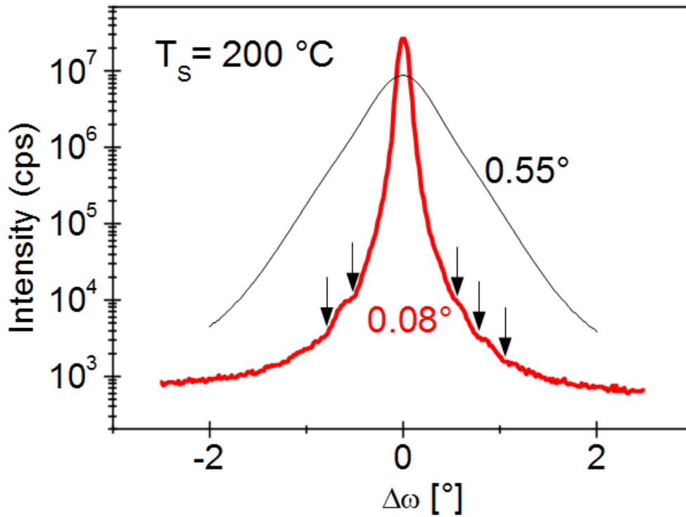
**Figure 2:** XRD curves of the (-220) reflection of GaAs/Fe<sub>3</sub>Si core/shell NWs,  $T_s = 200^\circ\text{C}$ . A radial  $\omega 2\theta$ -scan (thick line) along the [-110] direction and an angular  $\omega$ -scan perpendicular to the [-110] direction (thin line), together with their full widths at half maximum (FWHM) are given. Thickness fringes are marked by arrows.
