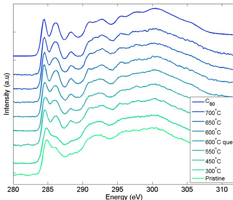
Figure 1: C K edge in different thermally annealed  $\text{Mg}_2\text{C}_{60}$  powders
