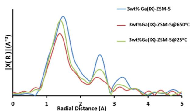
**Figure 6:** R-space spectra of 3wt%Ga(IX)-ZSM-5 showing the Ga environment in the sample as prepared, after reduction at  $650^\circ\text{C}$  and back at  $25^\circ\text{C}$ .
