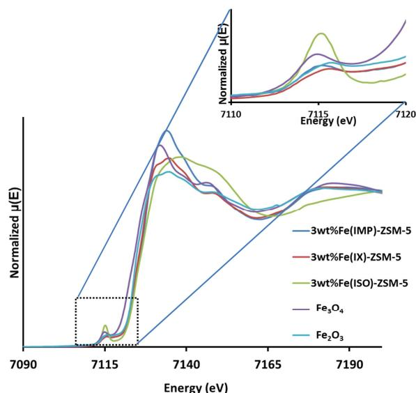
**Figure 2:** comparison of various XANES spectra of 3wt%Fe-ZSM-5 as prepared by various synthesis routes with the references  $\text{Fe}_2\text{O}_3$  and  $\text{Fe}_3\text{O}_4$ . Inset: zoom of the pre-edge features of the samples.
