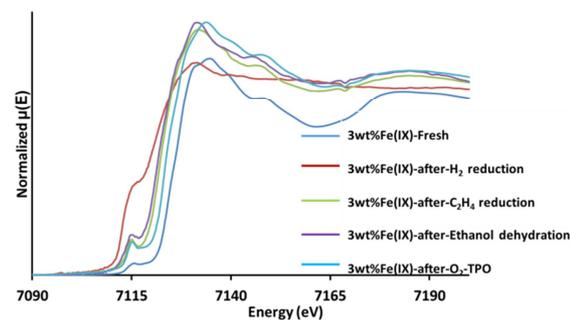
**Figure 3:** The XANES profiles of the 3wt%Fe(IX) samples after various reactive treatments.
