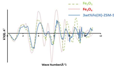
**Figure 4:**  $k^2$  weighted spectra of references and reoxidized 3wt%Fe(IX)-ZSM-5
