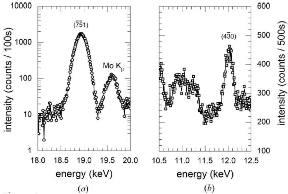
Figure 1: Determination of the energy of Bragg reflections with an energy dispersive point detector (a) the  $\bar{7}51$  fundamental reflection ( $\gamma + \gamma'$  phases) and (b) the 4-30 superstructure reflection ( $\gamma'$  phase only).
