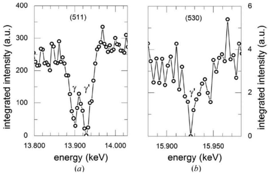
Figure 2: Determination of the energy of Bragg reflections with the Rainbow method (a) the 511 fundamental reflection ( $\gamma$  and  $\gamma'$  phases) and (b) the 530 superstructure reflection ( $\gamma'$  phase only).
