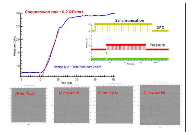
Figure 1: Typical measurements made during a compression rampe. Structural evolution of water in ramp n°8. The compression rate achieved was 0.2 GPa/ms.
