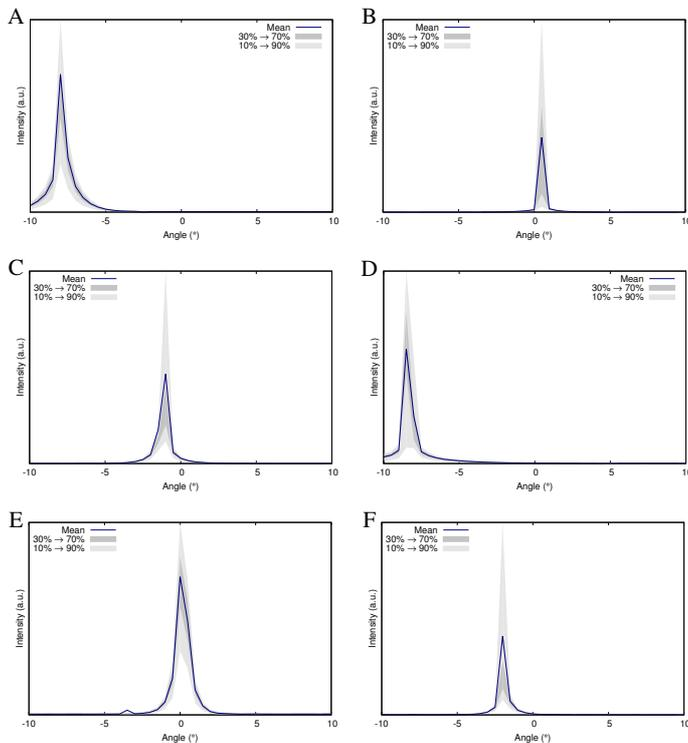
Figure 4: Rocking curves of various reflections from the  $0.5^\circ$ -interval rotational scan. A: (110), B: (113), C: (116), D: (118), E: (119), F: (125).
