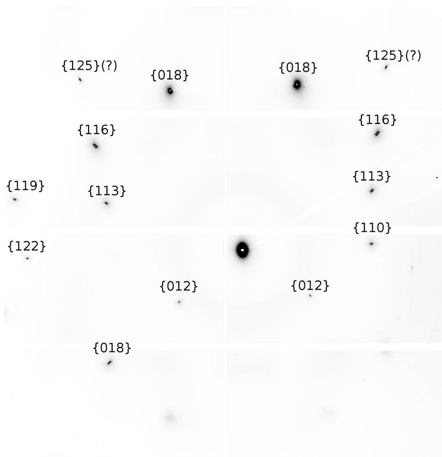
Figure 2: An averaged image from all the studied rotations (from a rotational line scan), with markings of the observed reflections.
