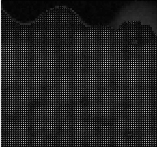
Figure 3: Large area scan, map of (113) plane. Evidently, all the peaks are at the same azimuthal/radial location, although they vary in intensity.
