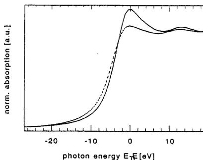
Fig. 2 Comparison of the XANES at the Pt  $L_3$  edge with and without scattering filter. BN sheets were added to a Pt metal foil to enhance diffuse scattering.
