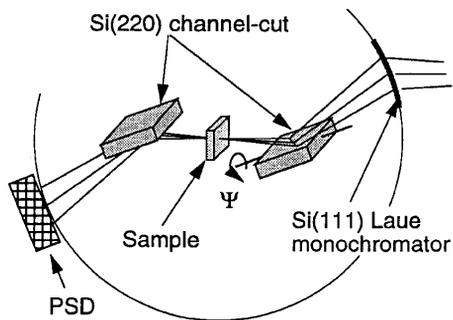
Fig. 1 Top view of the energy dispersive XAFS set-up using a filter for small angle scattering. The two Si(220) crystals arranged in the Bonse-Hart configuration are rotated by an angle  $\gamma$  in order to match the dispersion of the curved Laue monochromator.
