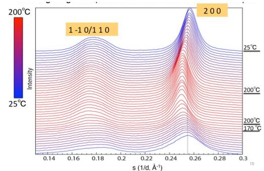
Figure 2 . WAXS equatorial profile of beech with 130% water content during annealing
