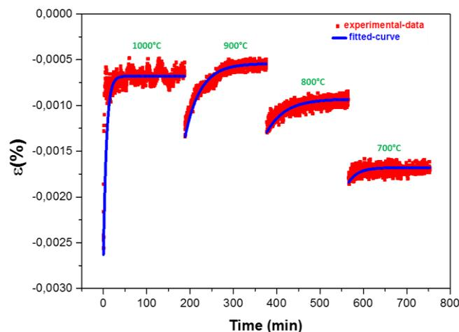
Fig. 2 : Internal strain evolution as a function of the oxidation time, for four subsequent plateaus of 3 hours, at respectively 1000, 900, 800 and 700 °C. The three later are observed after low-temperature jumps of 100°C. The microstructure has been built initially at 1000°C during the first plateau (no more significant evolution of the intensity or the width during the subsequent plateaus at lower temperatures)
