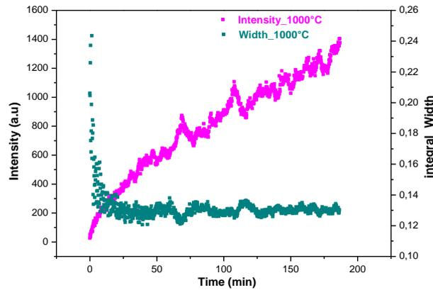
Fig. 1 : Intensity and integral width evolution for a chromia microstructure built at 1000°C on NiCr during a first plateau of 3 hours.
