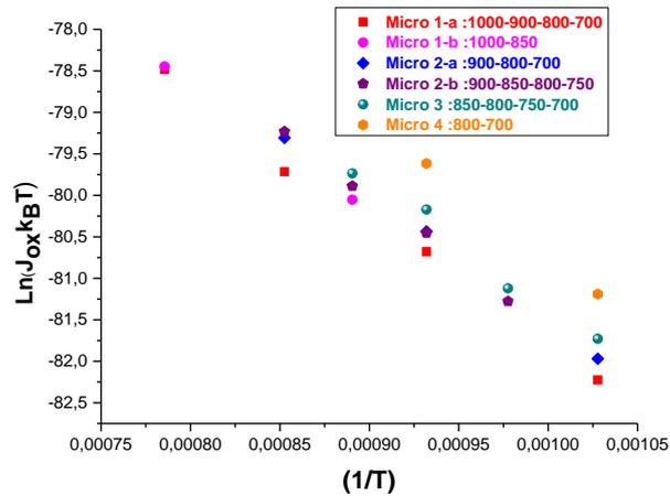
Fig. 3 : Creep coefficients  $J_{ox}$  as a function of the oxidation temperature, for the four initially built microstructures at respectively 1000, 900, 850 and 800°C. Both the initial building temperatures and the ones corresponding to the subsequent plateaus after the jumps are reported.
