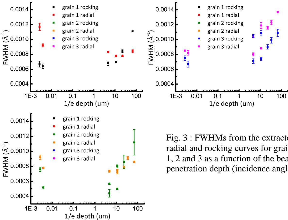
Fig. 3 : FWHMs from the extracted radial and rocking curves for grains 1, 2 and 3 as a function of the beam penetration depth (incidence angle).
