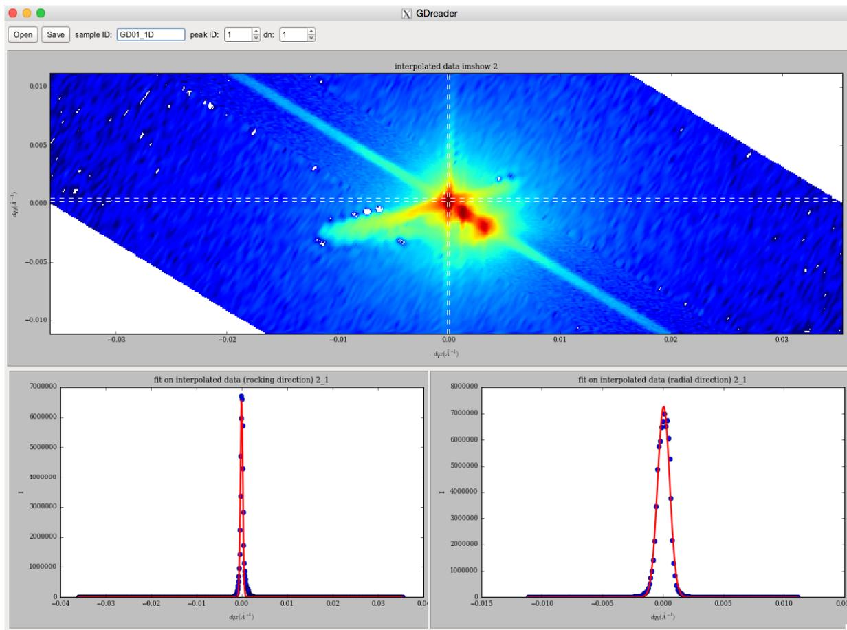
Fig. 2 : The program used to reconstruct the in-plane intensity map and to fit the extracted radial of rocking curve.
