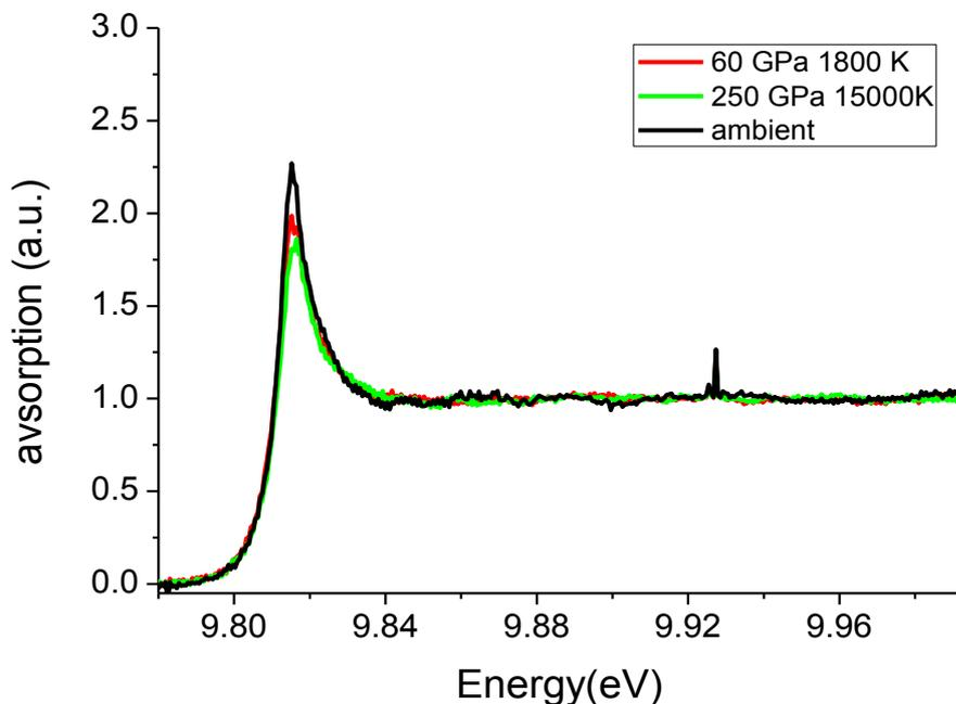
Figure 1: Effect of shocked state on the XANES spectra. Spectra were obtained with 1 x-ray bunch.
