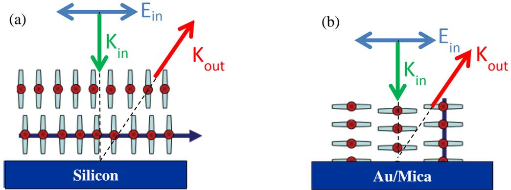
Figure 2: Normal incidence scattering geometry of the RIXS measurement for (a) FePc and (b) CoPc.
