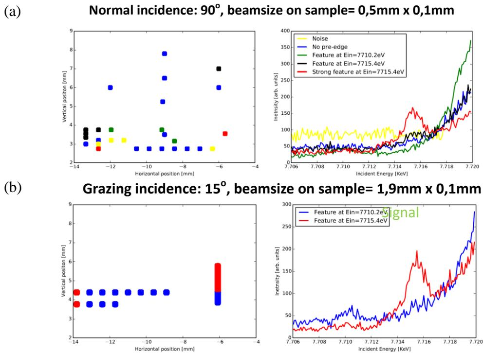
Figure 7: (a) Normal incidence measurement: Left graph shows the different sample spots that were measured probed, the colour of the spot correlated to the type of pre-edge observed. Right graph shows the different pre-edge features observed at different positions of the sample and (b) for grazing incidence.
