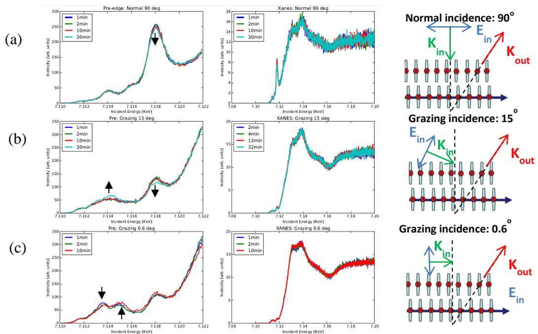
Figure 3: Radiation damage assessment for the FePc thin films. (a) HERFD measured at normal incidence, (b) and (c) at grazing incidence of angles  $15^\circ$  and  $0.6^\circ$  as shown at the right side.
