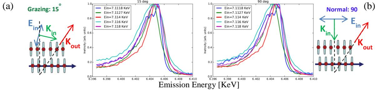
Figure 5: Fe 1s2p RXES slices measured at different incidence energies. (a) grazing and (b) normal incidence configuration.
