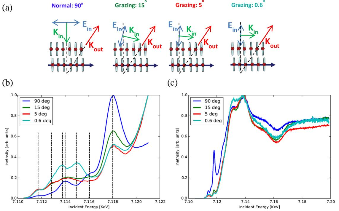
Figure 4: HERFD-XANES of FePc thin film as a function of angles. (a) shows the geometries used for the measurement from normal to grazing incidence. (b) is a zoom of the pre-edge region and (c) shows the full range.
