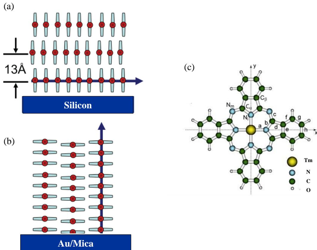
Figure 1: Samples measured at the beamtime. (a) sketch of FePc thin film, (b) of CoPc and (c) TmPc molecule.
