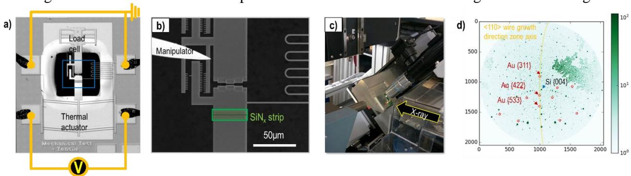
Figure 1. a) Thermally actuated nanotensile stage b) and the close up view. c) Sample mounted at BM32 d) CCD image of Laue pattern of the Au nanowire. Red is indexed Au peaks and the  $\langle 0-11 \rangle$  wire zone axis is labeled in yellow line.
