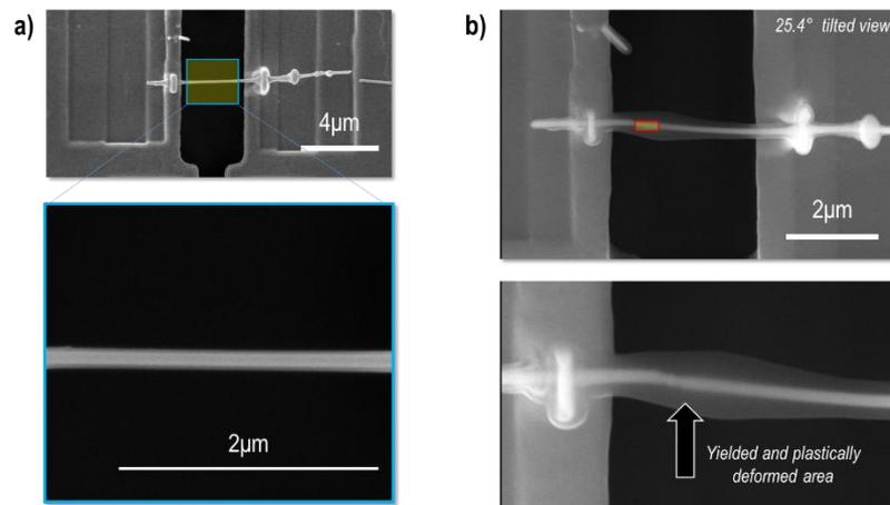
Figure 4. a) SEM image of the nanowire before and b) after the in situ tensile tests at ID01. The rough beam size and the position is marked in red squared box.
