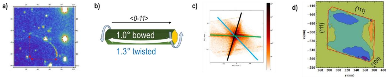
Figure 2. a) Sum of {311} peak along the wire measured in BM32 b) schematic of as-manipulated nanowire understood by the micro-Laue analysis c) {311} Bragg peak measured in ID01 before straining d) 2D reconstruction of the wire
