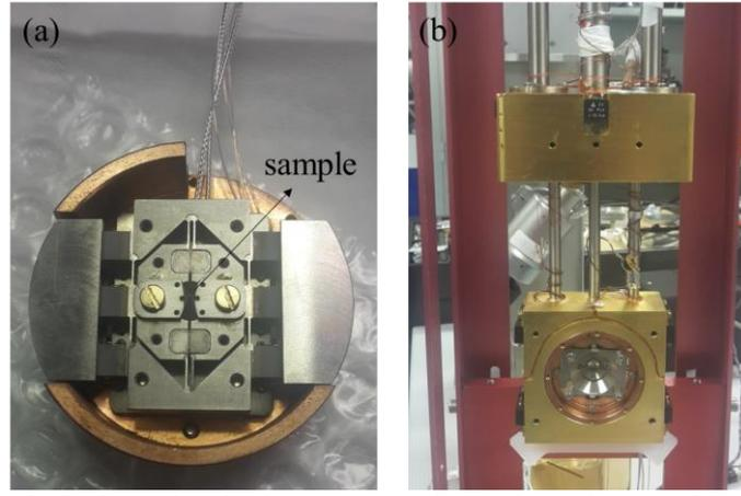
Fig. 1: (a) The piezoelectric based strain device mounted on the adaptor ring of the cryostat. The sample position in indicated. (b) The device mounted on the continuous flow He-cryostat of ID28.
