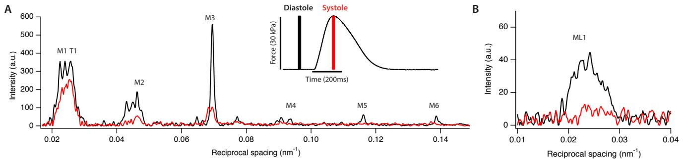
**Fig. 1** Meridional intensity profiles (A) and intensity profiles of the first myosin layer line reflection (B, ML1) from patterns collected during diastole (black trace) and systole (red trace, see inset). FReLoN detector at 1.6m camera length. Data from one trabecula; exposure time, 40ms. Temperature, 27°C; stimulation frequency, 1 Hz.
