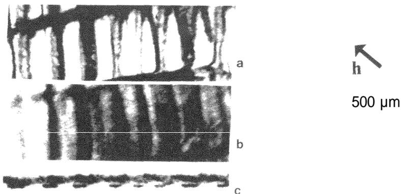
Fig.1: Monochromatic beam tomographs ( $\lambda \cong 0.3 \text{ \AA}$ ) recorded during the heli-ferromagnetic phase transition in a 0.4 mm thick (010) MnP, performed by using the a) 220 reflection from a steady silicon monochromator b) same, but vibrating monochromator. A section topograph corresponding to the case a) is shown on c: it indicates that the ferromagnetic regions are mainly located in the neighbourhood of the surfaces.
