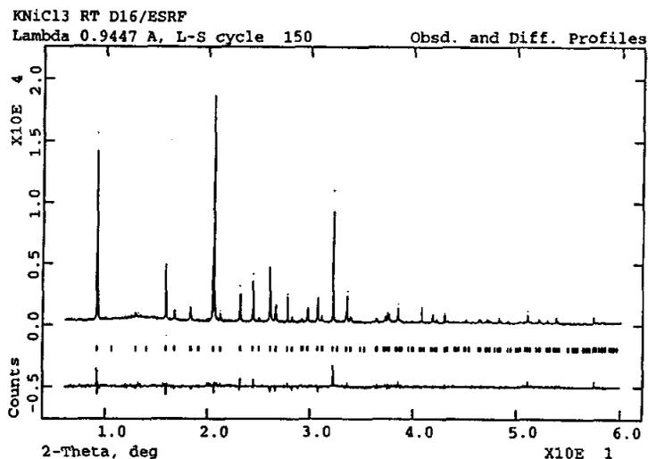
Fig.1 Diffraction Pattern of KNiCl<sub>3</sub> at 290K fitted with the GSAS code.
