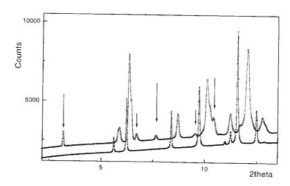
Fig. 1 Diffraction patterns of  $UPd_2Al_3$  below (full circles) and above (open circles) the structural phase transition at  $p \approx 250$  kbar. Arrows indicate additional reflections of the high pressure phase.
