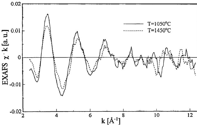
Fig. 1 k-weighted EXAFS spectra of levitated liquid Co<sub>80</sub>Pd<sub>20</sub> at temperatures of 1450°C and 1050°C.
