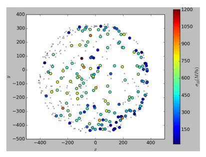
Figure 3. Radial positions and stress state of individual grains in the sample "R117-680".
