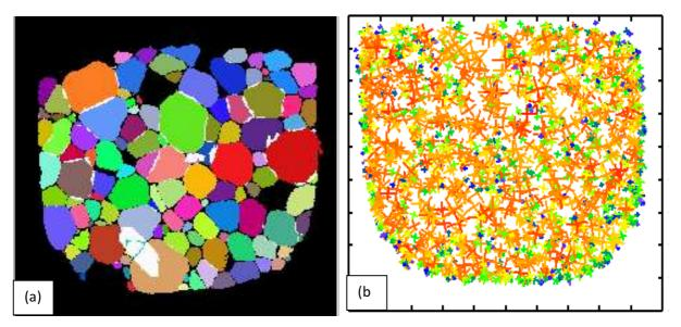
Figure 1. Unstrained AH35 sample containing more than 1400 grains in the probed volume: (a) DCT reconstruction, (b) 3DXRD result.
