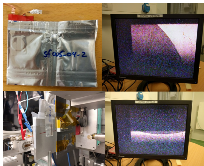
Figure 2. (top left) Planar pouch cell. (top right, bottom right) X-ray eye is able to observe the edge of the electrode. (bottom left) Pouch cell mounted in beam path and connected to portable potentiostat
