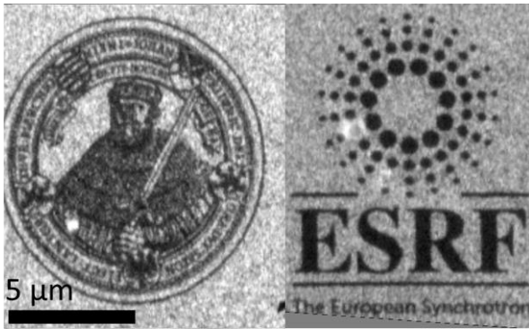
Figure 2: Greyscale heatmap of the unmodified (020)_{M1} Bragg peak for exemplary structured irradiation patterns.
