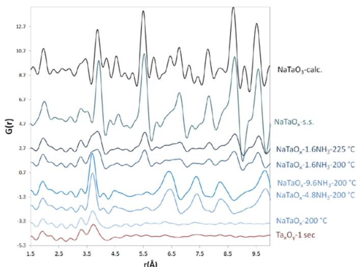
**Fig.3b.** PDFs obtained for  $\text{NaTaO}_x$  samples synthesized under different conditions vs. reference  $\text{NaTaO}_3$ <sup>[4]</sup>. Amounts of  $\text{NH}_3$  used in the synthesis are in mL. The PDF for  $\text{Ta}_x\text{O}_y$  (injection time of 1 sec) is added for comparison.
