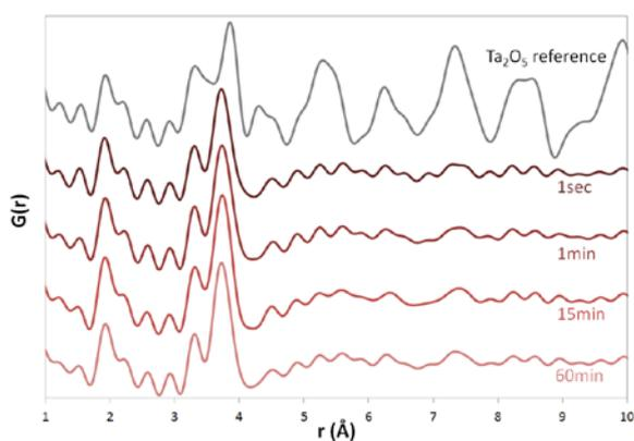
**Fig.3a.** PDFs obtained for  $\text{Ta}_x\text{O}_y$  samples synthesized with different injection times of the precursor vs. reference  $\text{Ta}_2\text{O}_5$ .
