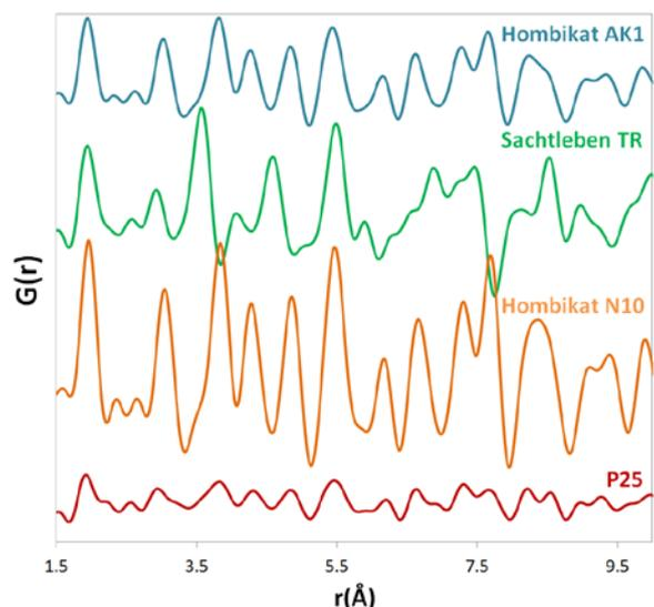
**Fig.1a.** PDFs of crystalline  $\text{TiO}_2$  powders. Hombikat AK1 consists mainly of anatase, Sachtleben TR consists of rutile, P25 and Hombikat N10 are mixtures of anatase and rutile structures.
