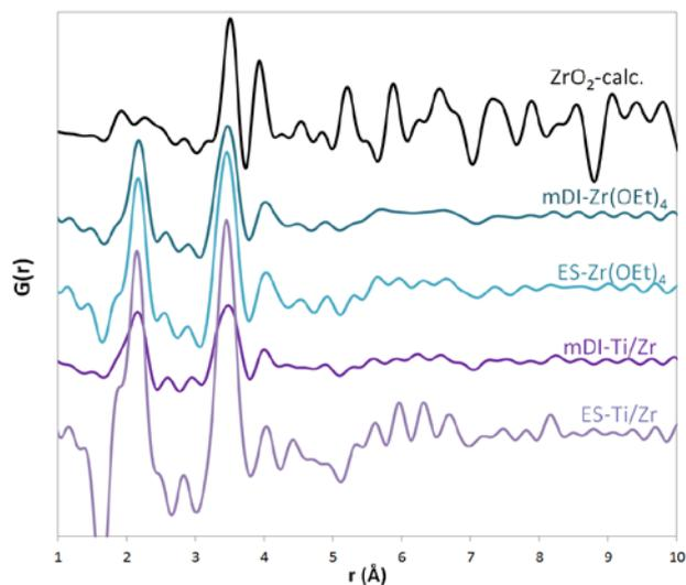
**Fig.4.b.** PDFs obtained for  $\text{ZrO}_x$  samples synthesized by direct injection (mDI- $\text{Zr}(\text{OEt})_4$ ) and *ex situ* methods (ES- $\text{Nb}(\text{OEt})_5$ ). The figure shows also the PDFs of Ti/Zr mixed oxides synthesized by *ex situ* and direct injection methods. 'm' denotes mixing the precursor in methanol before injection.
