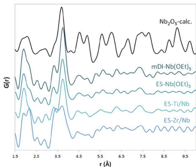
**Fig.4.a.** PDFs obtained for  $\text{Nb}_x\text{O}_y$  samples synthesized by the direct injection (mDI- $\text{Nb}(\text{OEt})_5$ ) and *ex situ* methods (ES- $\text{Nb}(\text{OEt})_5$ ). The figure shows also the PDFs of *ex situ* synthesized Ti/Nb and Zr/Nb mixed oxides. 'm' denotes mixing the precursor in methanol before injection.
