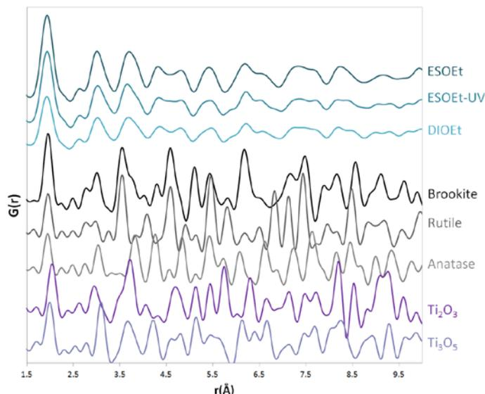
**Fig.1b.** Comparison of PDFs obtained for  $\text{TiO}_2$  samples synthesized *ex situ* with UV light irradiation and via direct injection method with calculated PDFs of the polymorphs of  $\text{TiO}_2$  and different titanium oxides.
