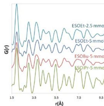
**Fig.2.** PDFs obtained for  $\text{TiO}_2$  samples synthesized using different precursor concentrations and precursor compositions.
