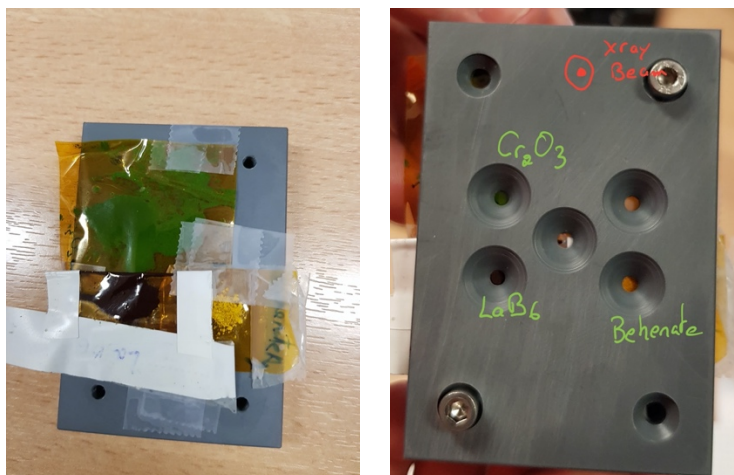
Fig. 2. Standards for alignments mounted on a pouch cell holder
