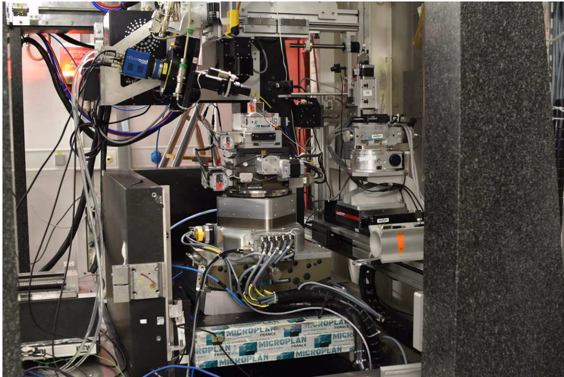
Fig. 5: Photograph of the in situ setup with sample T5 mounted into Nanox and installed on the ID11 diffractometer.
