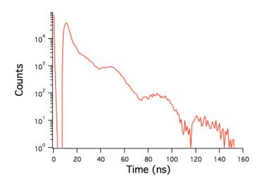
Time resolved NRS spectrum of 0.3 ML of Sn on Si(111) at about in grazing incidence and forward scattering conditions
