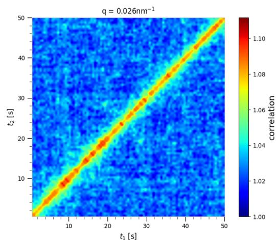
Figure 2: Two time correlation function measured with an unirradiated OMCA-CTAB sample with 100nm NP. The incoming intensity was attenuated by a factor of hundred.
