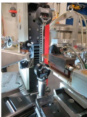
Drawing from one side (upper clamp) Localized heating (hot shoe)
