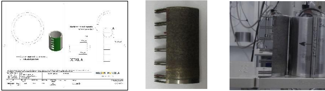
Figure 2: d_0 specimen machined by EDM wire cutting and set-up on beam line.
