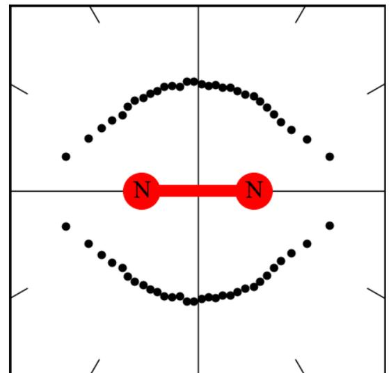
Fig. 2 – Molecular-frame Compton electron angular distributions. The Compton distribution clearly follows the molecular axis.
