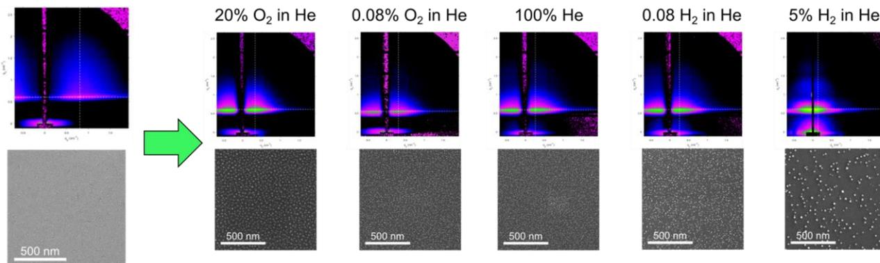
**Figure 2:** SEM images and GISAXS patterns for the starting sample and after annealing under different atmospheres. The surface has changed under all annealing conditions. However, the largest difference occurs for the 5% H<sub>2</sub> in He atmosphere.
