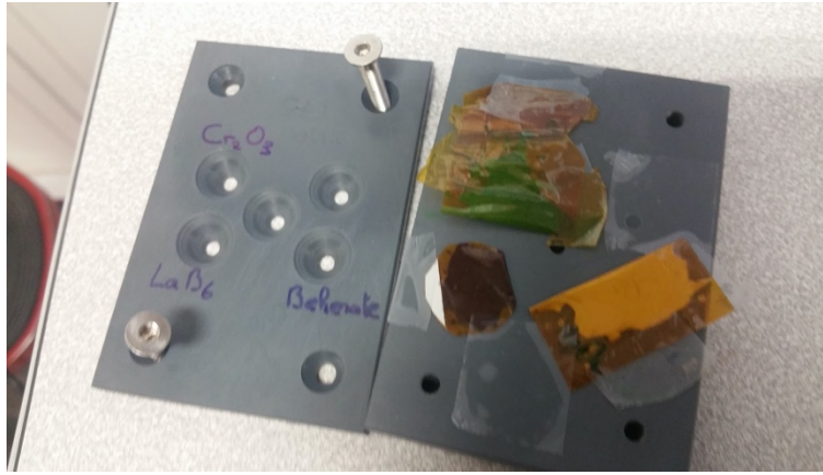
Fig. 2. Standards for alignments mounted on a pouch cell holder
