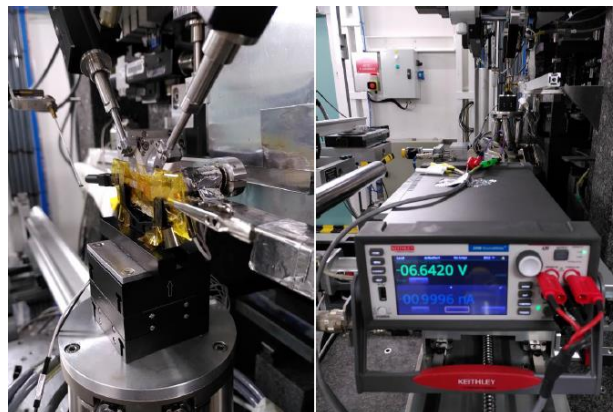
Fig. 12: A new setup to cycle solid state battery was tested at the ID13 (beamtime May 2022/II).
