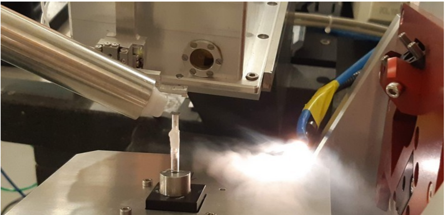
Figure 2: View of the sample on its capillary, with the nose of the cryostream. The incident beam aperture is visible behind.
